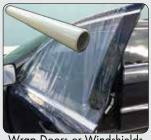
Wrap Doors or Windshields when glass is damaged
