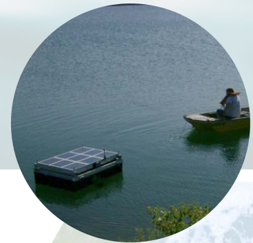
ULTRASONIC PONTOON INSTALLED IN RESERVOIR 1
