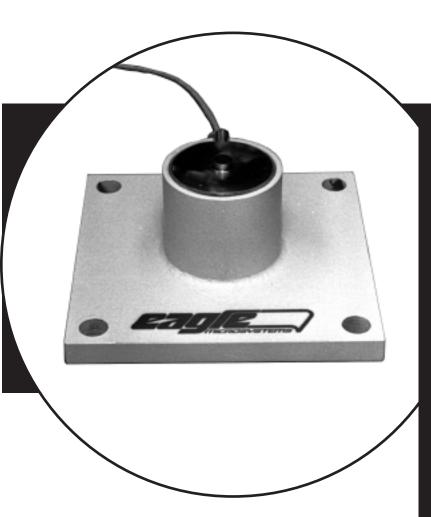
The Eagle Microsystems Model HC3600/7200 Hydraulic-to-Electronic Conversion Assembly is an electronic load cell replacement for hydraulic load cells used in ton container scales. The assembly has no moving parts and is immune to drifting problems associated with hydraulic load cells. Used with Eagle digital instrumentation the assembly inherently provides the capabilities of:
