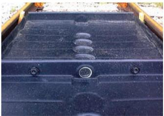
Large, 3"-diameter flow-through channels allow spills to quickly travel from one Pan to the next. Channels are located at the low point in each Center and Side Track Pan.
